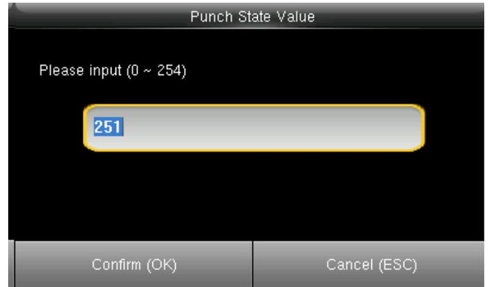
You can change the punch state value by entering into the input section using the keypad.
