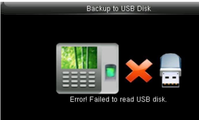
If the usb is not properly inserted the above screen will be displayed. You can either change the USB or insert it properly again.
