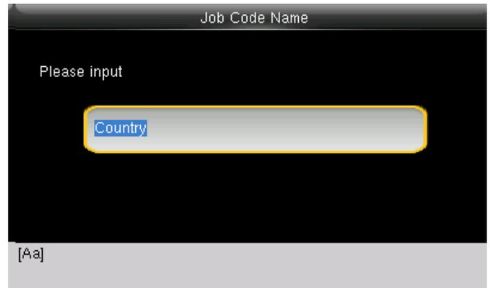
To change the job group name to country as shown above we need to press\* key to switch the input method and type country using the keypad.
