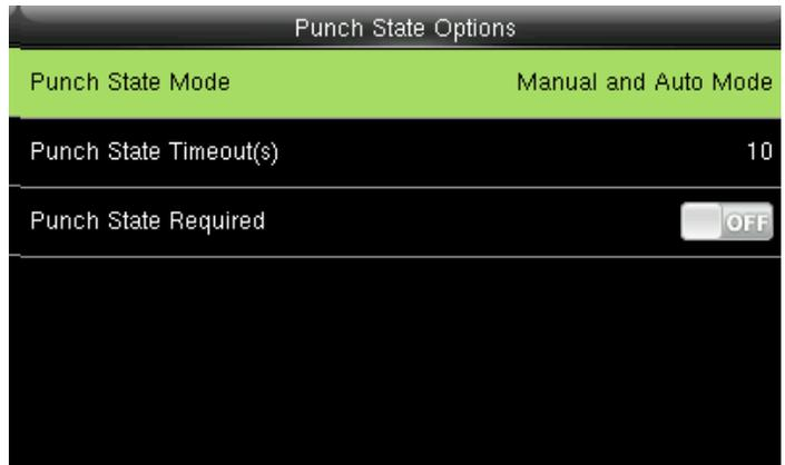
Press to select items. When the setting is completed, press **OK** to save the setting and exit.
