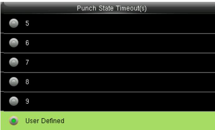
You can change the punch state timeout from the image above. The timeout ranges from 5 to 99 sec.
