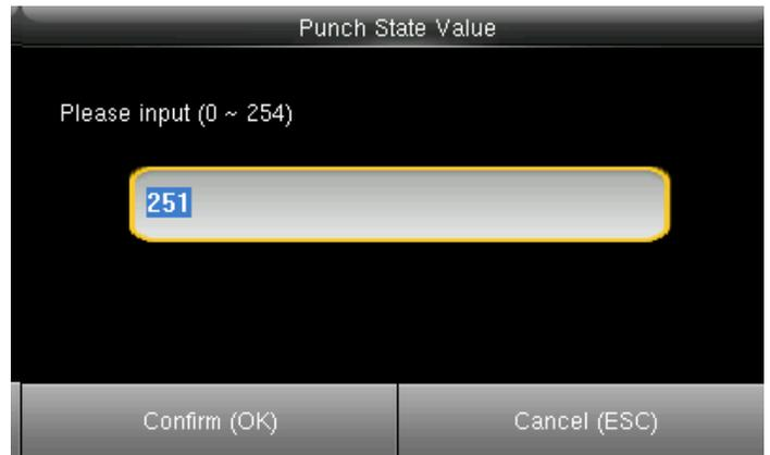
You can change the value of the punch state by changing the value in the input screen with the help of keypad.
