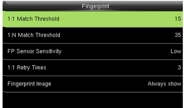
Here select **1:1 match threshold** The value is similar to the ID+fingerprint verification and the enrolled template.
