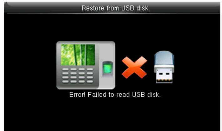
If the USB disk is not properly inserted the above screen will be displayed. You can either change the USB or insert it properly again.
