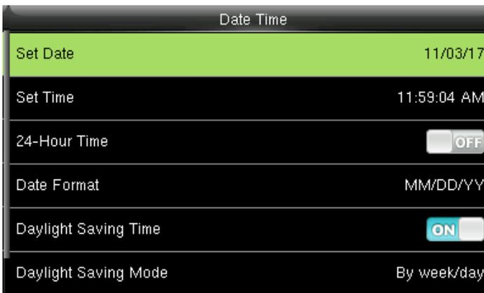
Select items. When the setting is completed, press **OK** to save the setting and exit.
