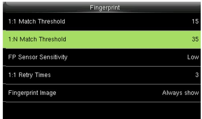
Here select **1:N match threshold** The value is similar to verification and the enrolled template.
